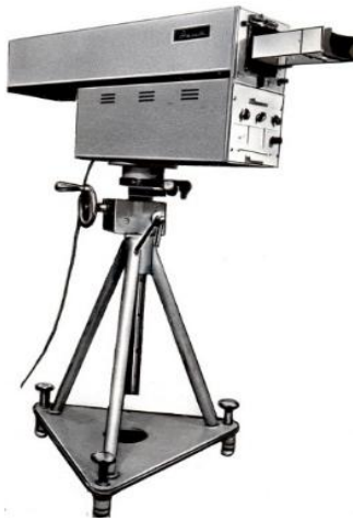
Fig. 4. Camera Agat-SF1 on a support: size 903x202x388 mm, weight of 30 kg, power consumption 100 VA.
