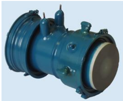
Fig. 5. Miniature PV-201 streak tube, used in the K008 camera (has one MCP): photocathode S20, length 78 mm, width/diameter is 60/48 mm, weight 0.45 kg.
