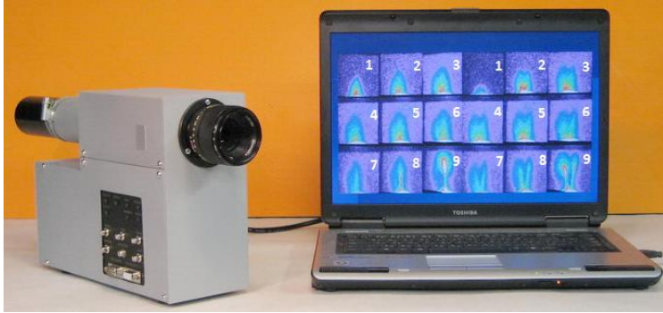
Fig. 11. K011 camera: dimensions: 350x120x220 mm, weight: 4 kg, power consumption \leq 20 VA, CCD camera RU-05M – 1392x1032 pixels, ADC – 12 bits.
