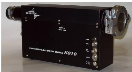
Fig. 9. K010X camera: dimensions: 440x120x205 mm, weight: 5.5 kg, power consumption \leq 10 VA, RU-05M camera (5) – 1392x1032 pixels, ADC – 12 bits.
