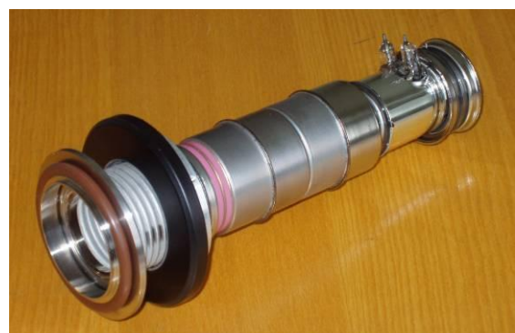
Fig. 10. Open (pumpable) PV-204XM streak tube, which is used in K010X camera (has one MCP): slit and frame CsJ and Au photocathodes are removable, length 215 mm, width/diameter 75/75 mm, weight 0.75 kg.
