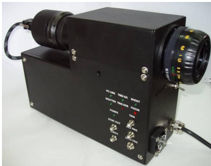
Fig. 8. K008Smart camera: dimensions: 305x85x195 mm, weight: 3.6 kg, power consumption \leq 20 VA, new compact RU-05R CCD camera – 1392x1032 pixels, ADC – 12 bits.
