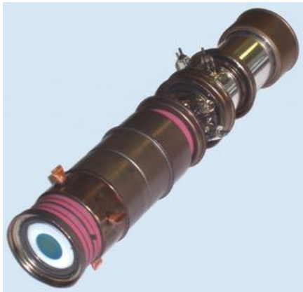
Fig. 13. PV-206 streak tube without MCP, which is used in K016 camera: photocathode S1 or S20, length 240 mm, width/diameter 69/48 mm, weight 0.9 kg.
