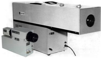
Fig. 7. Streak cameras of the second and third generations. Right: Agat-SF1 camera: 2 ps limiting temporal resolution, photofilm image recording; dimensions 903x202x388 mm; weight: 30 kg; power consumption 100 VA. Left: the first model of K008 camera: 50 ps limiting temporal resolution, dimensions 335x90x190 mm; weight 3.5 kg; power consumption 8.5 VA, RU-02M CCD camera – 582x500 pixels, ADC – 8 bits.
