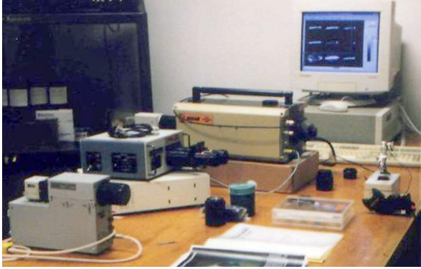
Fig. 1. The demonstration of apparatus. From left to right: K008 camera, PS001 photosensor and K004M camera. The electroshocker lies opposite the photosensor at the right on the brink of the desk.
