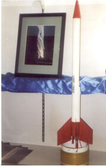
Fig. 1. A rocket of about 1 m length with a coil of wire on its tail used for lightning triggering
