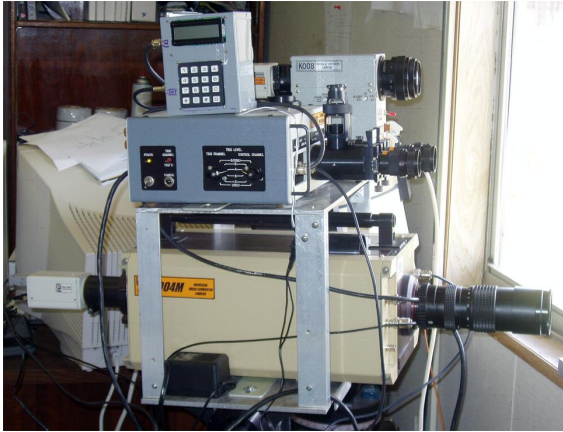
Fig. 11. The K004M camera is on a bottom platform of the stand; the K008 camera, the PS001 photosensor and the interlock are on an upper platform.
