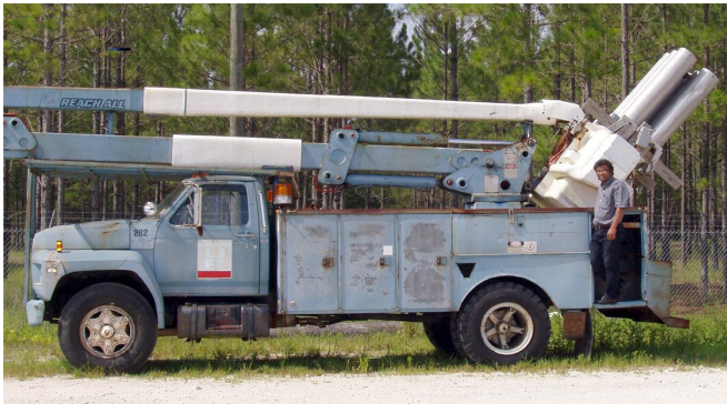
Fig. 3. A mobile 6-channel launcher
