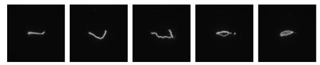
Fig. 9. Other different realization of discharge channel formation. Parameters of experiments corresponds to fig.6. The exposition – 10 ns. And the moment of exposition synchronizes to moment of maximum current at the first half-wave. High-speed camera – NanoGate-1. Spectral range of filming is 600-700 nm.
