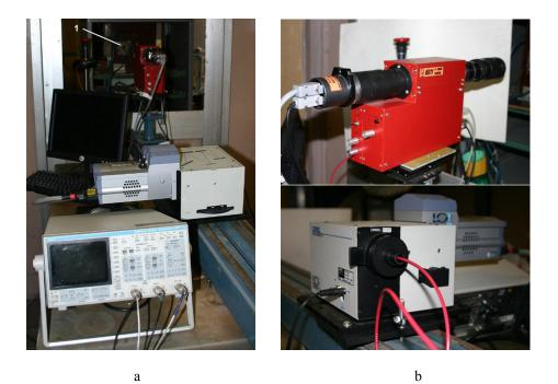
Fig. 3. General view of installation (a); 1 – discharge chamber. High-speed miniature 9-frame image converter camera K-011 (b - on high); imaging spectrograph MS127i with ICCD DH720-18F-03 (b – on down).
