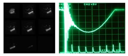
Fig. 7. Discharge evolution: Frames from left to right and from the top downward. On an oscillogram from above current pulse, from below frame pulses from high-speed camera (the impulse top corresponds to an exposure time, time between impulses to a pause between frames). The high-speed camera K-011. Maximum current ~ 35 A. Current rise rate  $\sim$ 5×10<sup>6</sup> A/s. Interelectrode gap 10 mm. I - current 10 A/div, time 2 µs/div.
