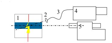
Fig. 2. Schematic drawing of diagnostic techniques: 1 – discharge chamber, 2 – collecting lens, 3 – fiber bundle, 4 - imaging spectrograph with ICCD, 5 - high-speed digital cameras.
