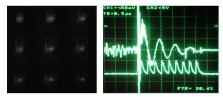
Fig. 5. Discharge evolution: Frames from left to right and from the top downward. On an oscillogram from above current pulse, from below frame pulses from high-speed camera (the impulse top corresponds to an exposure time, time between impulses to a pause between frames). The high-speed camera K-011. Maximum current ~ 30 A. Current rise rate ~ $10^8$  A/s. Interelectrode gap 10 mm. I - current 10 A/div, time 0.5 µs/div.
