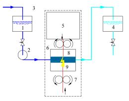
Fig. 1. The installation diagram. 1, 4 - tank with water, 2 - pump, 3 - electrodischarge block, 5 - high-voltage generator, 6 - electrodischarge chamber, 7 - feed mechanism of a spearhead electrode, 8, 9 - electrodes.
