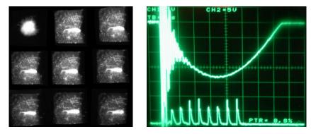
Fig. 8. Discharge evolution: Frames from left to right and from the top downward. On an oscillogram from above current pulse, from below frame pulses from high-speed camera (the impulse top corresponds to an exposure time, time between impulses to a pause between frames). The high-speed camera K-011. Maximum current ~ 40 A. Current rise rate  $\sim$ 5×10<sup>6</sup> A/s. Interelectrode gap 10 mm. I - current 10 A/div, time 2 µs/div.
