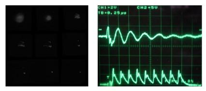
Fig. 6. Discharge evolution: Frames from left to right and from the top downward. On an oscillogram from above current pulse, from below frame pulses from high-speed camera (the impulse top corresponds to an exposure time, time between impulses to a pause between frames). The high-speed camera K-011. Maximum current ~ 40 A. Current rise rate ~ $10^8$  A/s. Interelectrode gap 10 mm. I - current 40 A/div, time 0.25 µs/div.
