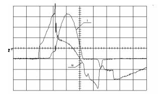
Fig. 4. Oscillograms of current and voltage on discharge impulse. I - current 10 A/div., U - voltage 400 V/div., time 10 µs/div.
