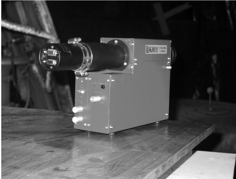
Fig. 2. K011 miniature programmable 9-frame image converter camera
