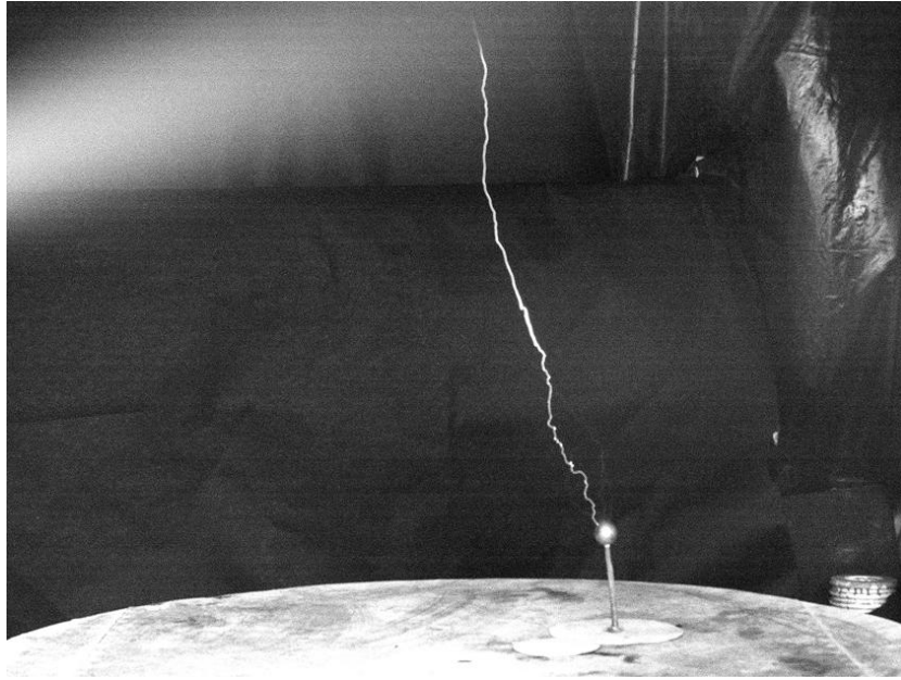
Fig. 8. Photograph of the final stage of the third type for discharge from an artificial charged aerosol cloud
