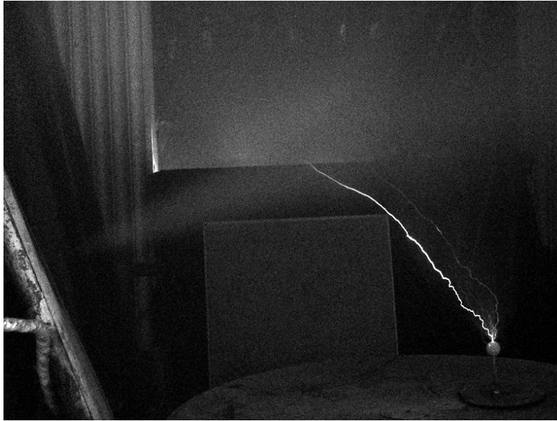
Fig. 3. Photograph of final stage of the first type for discharge from an artificial charged aerosol cloud.
