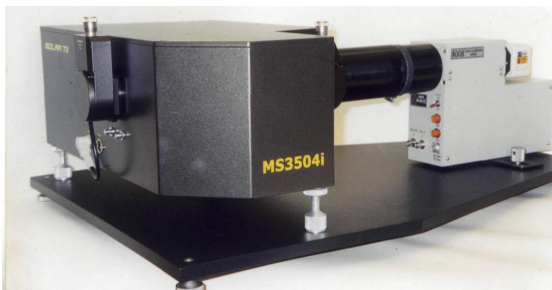
Fig.1. An appearance of the SVA-01 imaging temporal-analyzing monochromator/spectrograph.
